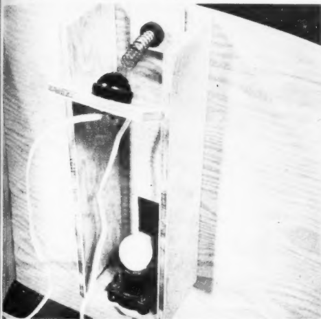
Light control detail. A dowel push rod bears against a doorbell push button to make exposure.
